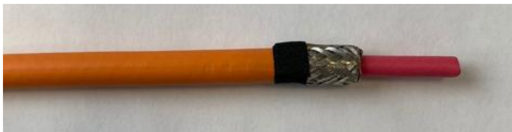
Figure 3.18: Representation 4.0 mm 2 SCC position protruded shielding braid (3.5 Fold over the shielding braid and secure the shielding braid)
