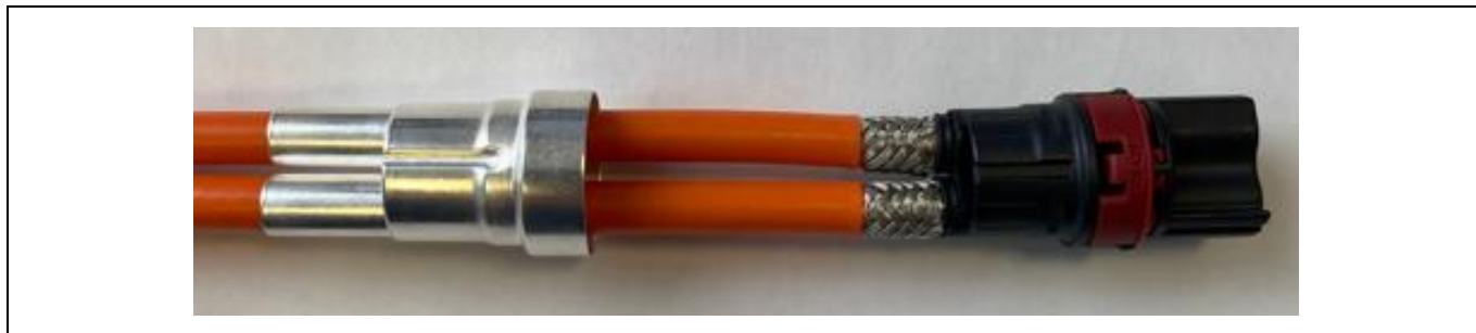
Figure 4.24: Representation 6.0 mm² SCC protruded individual shielding strands (4.8 Slide the shielding sleeve onto the contact carrier)
