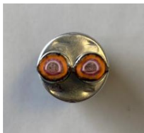
Figure 3.42: Representation 4.0 mm 2 SCC shielding sleeve fold (3.10.1 Cable shielding crimping using two half-shells)
