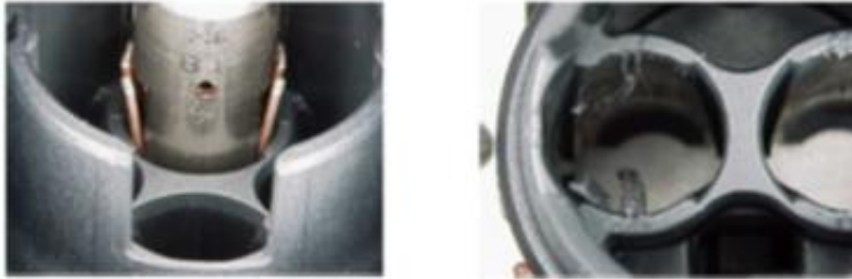
Figure 3.26: Representation 4.0 mm 2 SCC plastic burr on contact carrier (3.7 Inserting HCT4 female terminals into contact carrier)
