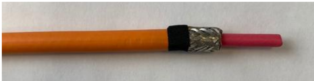
Figure 3.17: Representation 4.0 mm 2 SCC position fixing tape related to the ferrule crimp (3.5 Fold over the shielding braid and secure the shielding braid)
