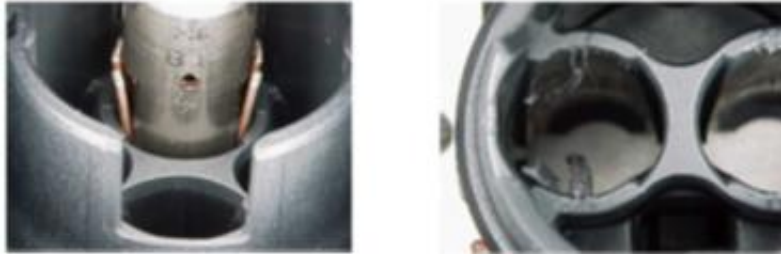
Figure 4.17: Representation 6.0 mm 2 SCC plastic burr on contact carrier (4.6 Inserting HCT4 female terminals into contact carrier)
