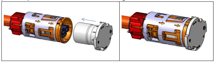
Insert the transport protection cap until both locking elements snap over the front collar of the connector housing. It is possible to turn the transport protection cap 360° during and after the assembling.
