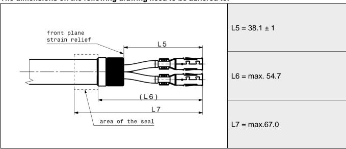
The dimension L5 is decisive for the position of strain relief. As alternative to L5 it is allowed to prove dimension L5.1. L6 is only for information and is built from L4.1 and L5. The dimensions are caused from L1, L4 and the EVS-100068 or L4.1 and L5.1.
