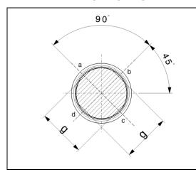
The dimension "g" results from the embossing in between a-c and b-d.
