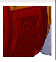
During closing the angled cap, make sure the wire insulation material doesn't get damaged. Take care that only the multi core cable is allowed under the angled cap. No Tape, protective tube, or other additional parts is allowed. All five latching hooks must be locked. Once the angled cap is closed, it is not possible to change the angle anymore.
