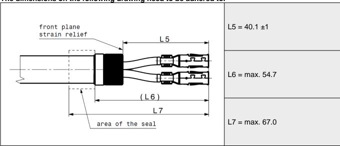
The dimension L5 is decisive for the position of strain relief. As alternative to L5 it is allowed to prove dimension 5.1, but one of the two combinations from L4.1 and L5.1 or L4 and L5 must be chosen. L6 is only for information and is built from L4.1 and L5. The dimensions are caused from L1, L4 and the EVS-100068.
