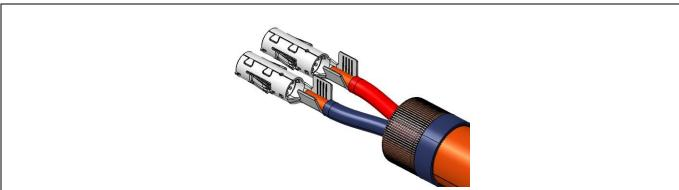
To do an orderly assembling / to ensure the primary locking and the secondary locking, the correct position of the terminals and the wire is very important and needs to be ensured. Usually, the horizontal version is intended.
