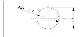
The plunger and anvil are pressed together until block. Due to this the dimension "d" will be given. See table of each cross section.
