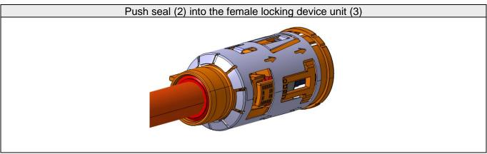
The cable seal can be slightly widened during assembly. It is possible to move the seal with the cover cap (1) on the wire, but care must be taken that the seal does not twist and is not pinched or damaged.
