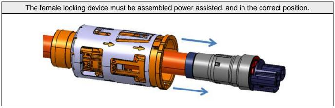
For the positioning and the assembling process of the female locking device unit onto the wire unit, the assembling device (Hand device) of the company "WKM" can be used.
