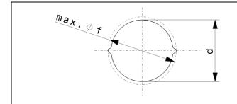
The plunger and anvil are pressed together until block. Due to this the dimension "**d**" will be given. See table of each cross section.
