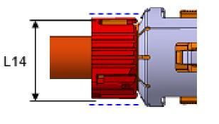
Do not damage the cover cap (1) or the seal (2) during assembly. If the cover cap is in end position the locking hooks on both sides must about straight on the female locking device unit. They are not allowed to stay in a deflected position. They must be within the dimension L14 = max. 25 mm
