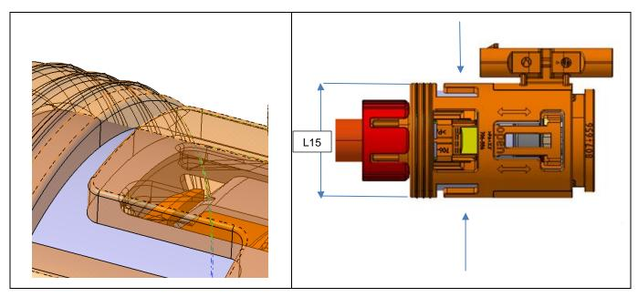
If the CPA Housing is in end position at least one of the locking hooks must about straight on the female locking device unit. They are not allowed to stay in a deflected position. They must be within the dimension L15 = max. 35.0 mm. Under certain circumstances (Tolerances) it needed to press on the locking hooks by hand.
