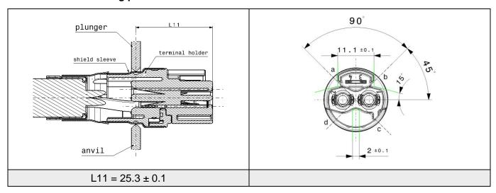
The dimension L11 describes the position of the pressing. The dimension L11 is considered as tool dimension and must be ensured in the tool.
