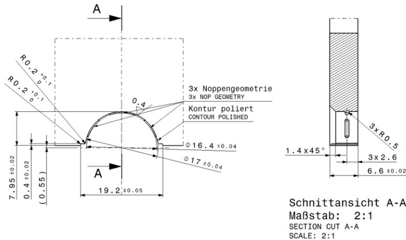
Anvil geometry of the wire shield pressing
