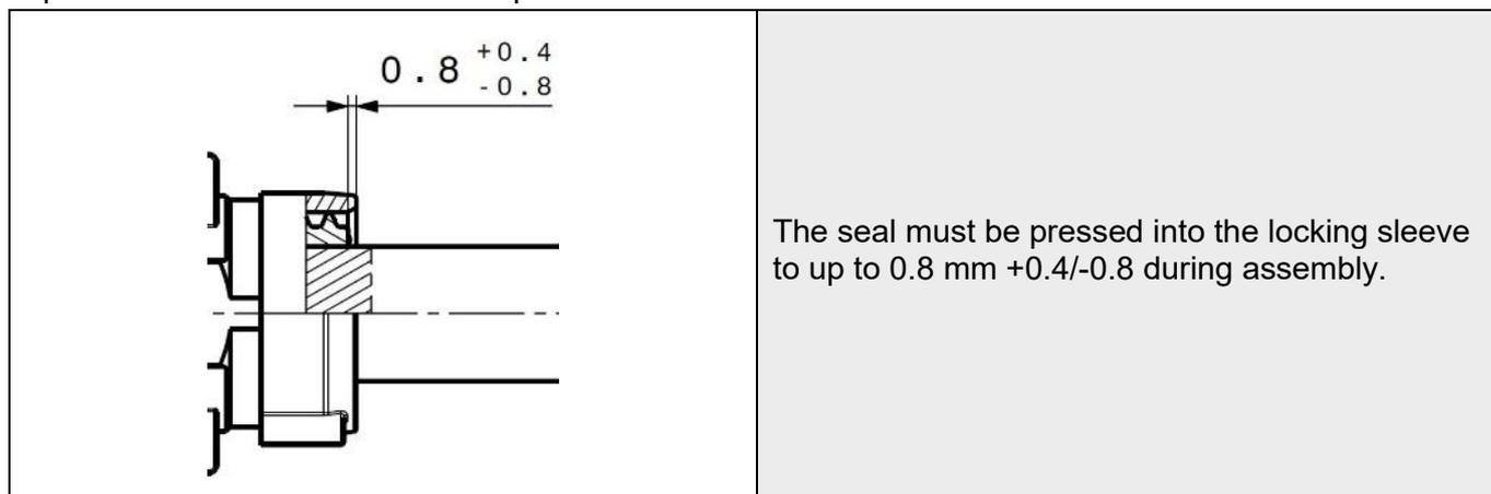
Connect the cover cap (5) over the recess provided in the locking sleeve (2). A press can be used for this assembly process. The holding of the retaining caps in the press, as well as the application of pressure, should take place over a surface that is as large as possible.
