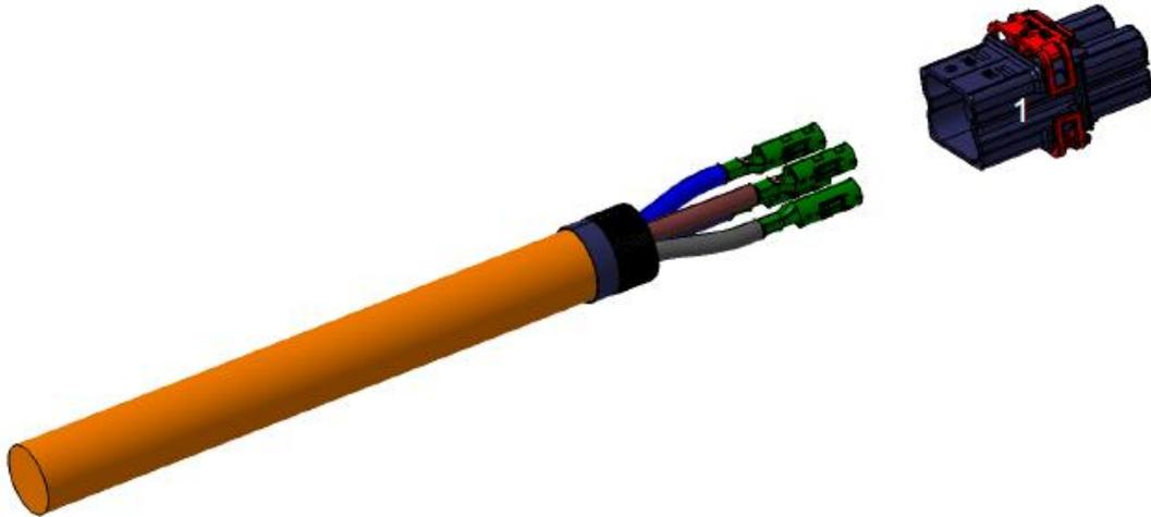
While assembling the HCT4 female terminals, the latching lance of the HCT4 female terminals will be deflected. Once the end position is reached, the latching lance will audibly engage, and the HCT4 female terminals will be primary locked (The HCT4 female terminals must be crimped).
