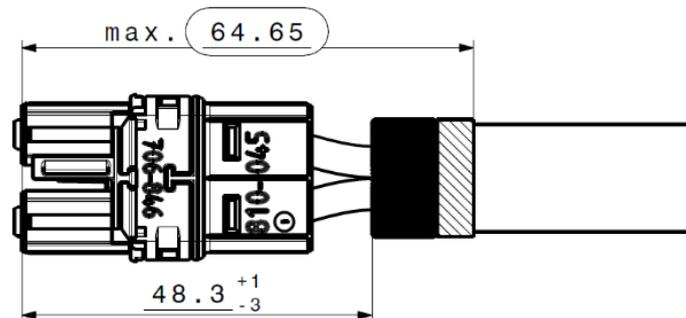
During measuring the dimensions  $48.3 \text{ }^{-3/+1}$  & max. 64.65 the contact carrier and the wire must be positioned in a suitable mounting fixture to correct the deviation of position of the contact carrier and the wire, if necessary.
