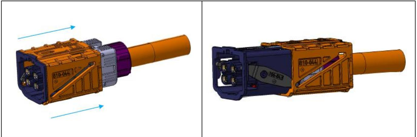
After assembling, the lever must be slide into end position.
