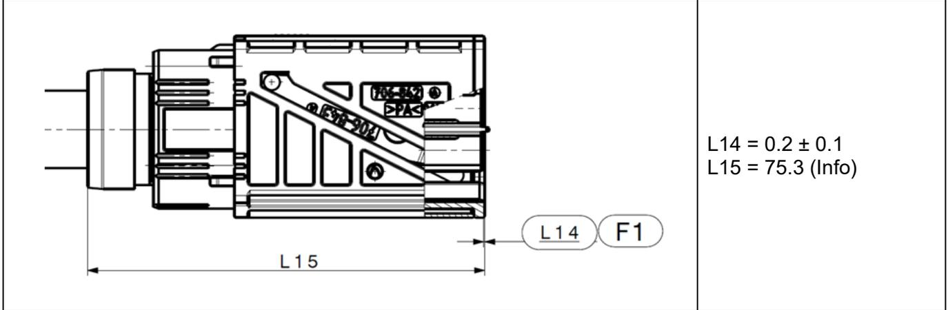
The locking sleeve must be assembled onto the shielding sleeve force assisted until the dimension L14 is reached.
