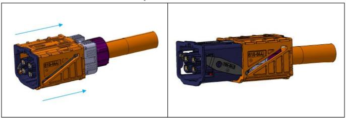
After assembling, the lever must be slide into end position.
