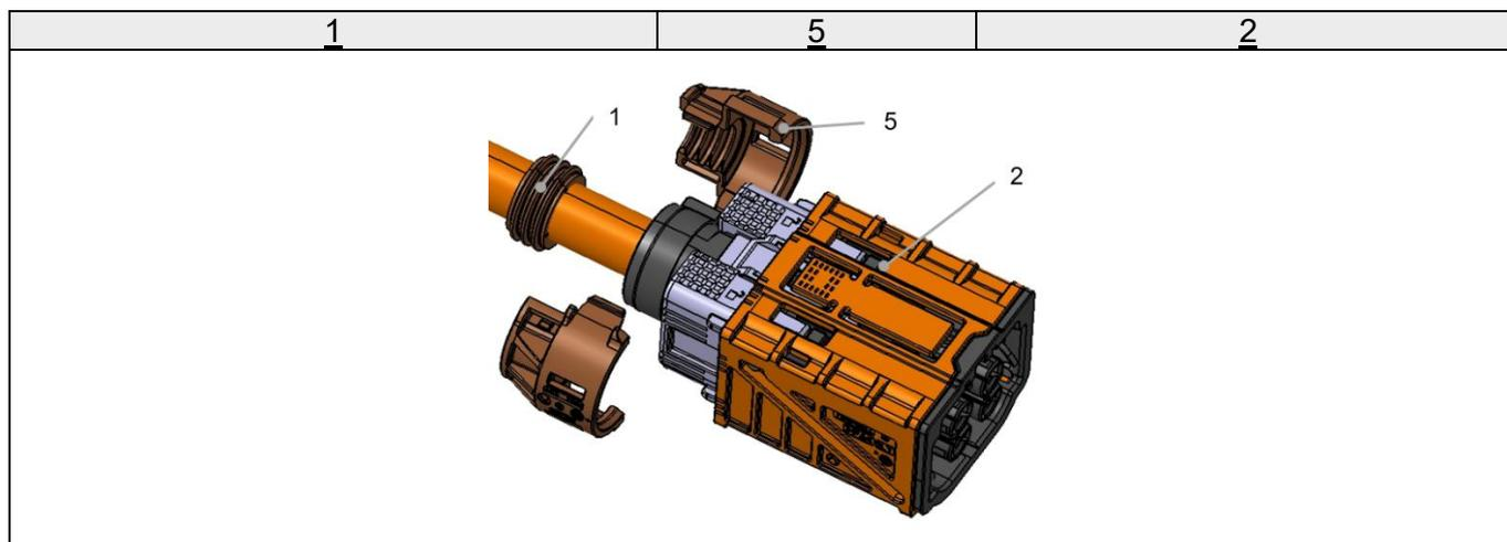
Slide the wire seal (1) into the locking sleeve (2)
