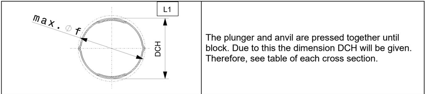
During the pressing process a fold appears on two sides. This fold is not allowed to be bigger than the diameter “f” = Ø 19.5 mm referring to the centerline of the wire. The diameter **DCH** must not be measured inside the embossing position but must be measured across the diameter.
