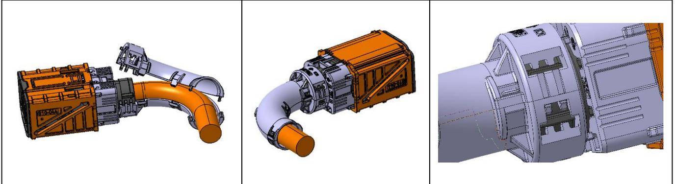
During closing the angled cap, make sure the wire insulation material doesn't get damaged. Take care that only the multi core cable is allowed under the angled cap. No Tape, protective tube, or other additional parts is allowed. All five latching hooks must be locked. Once the angled cap is closed, it is not possible to change the angle anymore.
