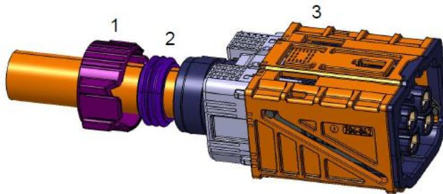
The wire seal can be slightly widened during assembly.
