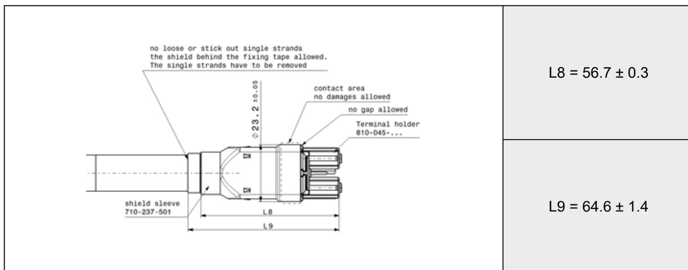
The dimension L8 and L9 are just for information. The dimensions are caused from the dimension L1, L4 and the EVS-100068.
